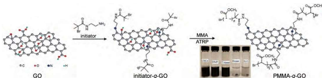
Figure 8. Preparation of PMMA-g-GO nanocomposites
