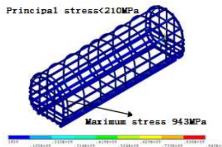
Figure 21. Overall stress cloud diagram of the solid model in nitrogen seal status
