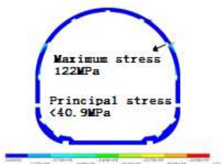
Figure 29. Arch beam stress cloud diagram of the solid model in lifting status
