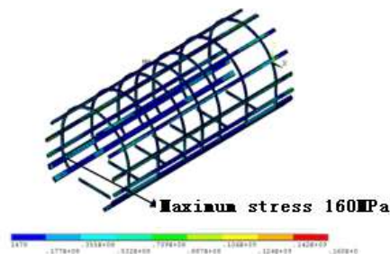
Figure 10. Overall stress cloud diagram of beam model in the test status
