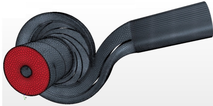
Figure 4. Calculated grid of screw centrifugal pump.
