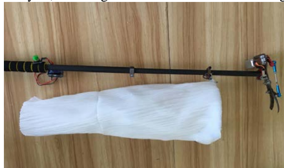
Figure 6. Structure of portable fruit picking device
