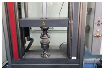
Figure 2. Zwick Z050 compression testing machine.
