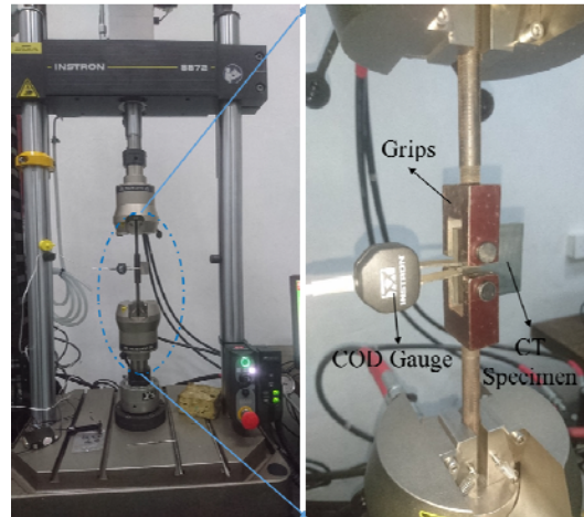
Figure. 4. Testing system setup for FCG
