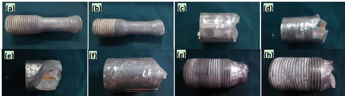
Figure 1. Fracture macro-profile of the bolts.
