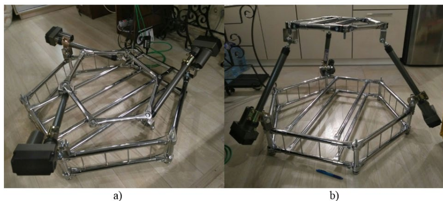
Figure 5. Prototypes of the robot with RRTRR (a) and RTS (b) joint structure.
