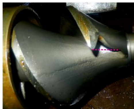
Figure 2. Erosion-corrosion of gas separator component.
