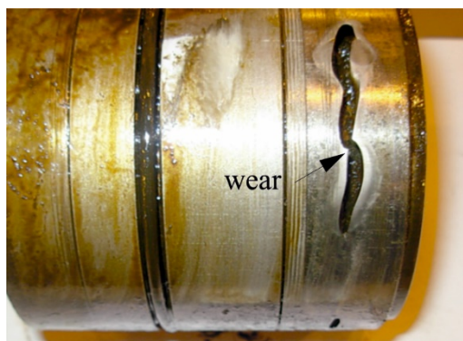
Figure 1. Erosion-corrosion of multistage centrifugal pumps component.
