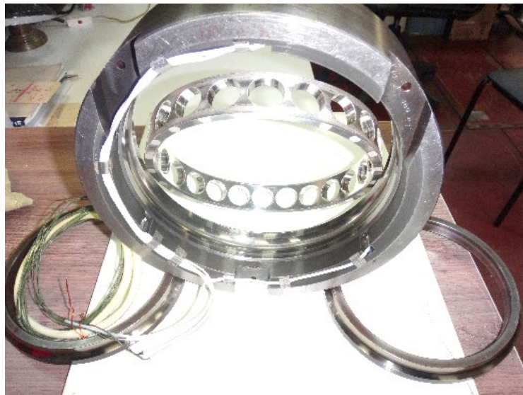
Figure 3. Installing the outer ring of bearing 126130 ( d = 150 mm) in the housing with the thermocouples on the outer ring.
