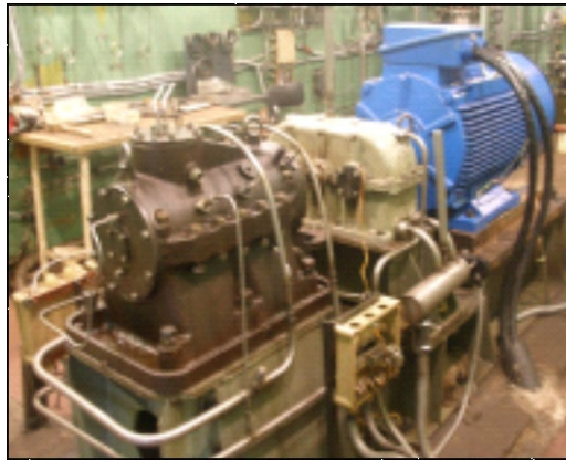
Figure 1. Bearing test rig T14–15/2.
