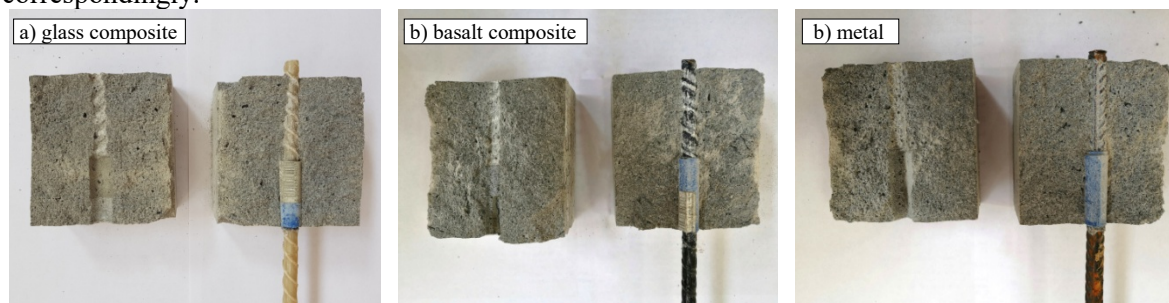
Figure 2. Nature of reinforcement elements cohesion failure with macroporous composite
