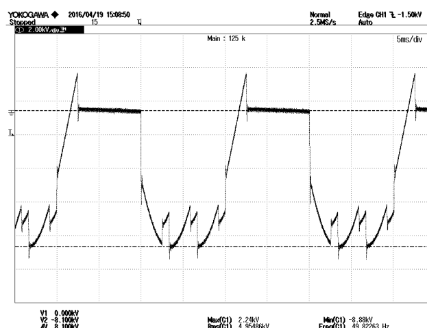
(a) Valve arrester aging test waveform of 6-pulse rectifier
