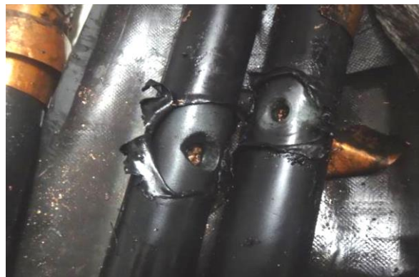
Figure 5. Cable insulation damaged point.
