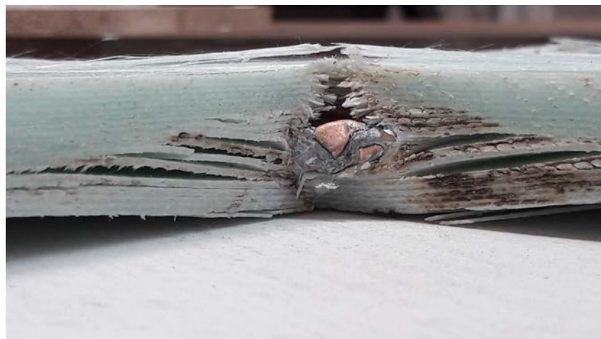
Figure 7. Composite glass fiber + resin, thickness of 13 mm, after the impact with 9 mm FMJ at 420 m/s [34]
