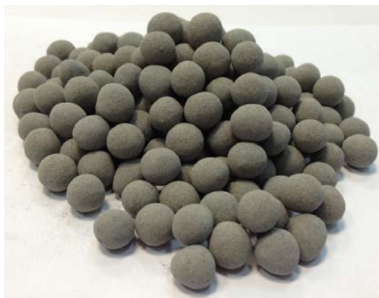
Figure 1. Non-fired fly ash gravel appearance.
