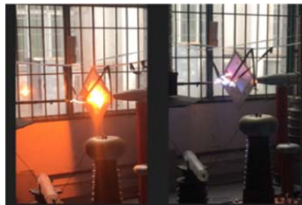
Figure 7. ZnS high voltage electric field test experiment.
