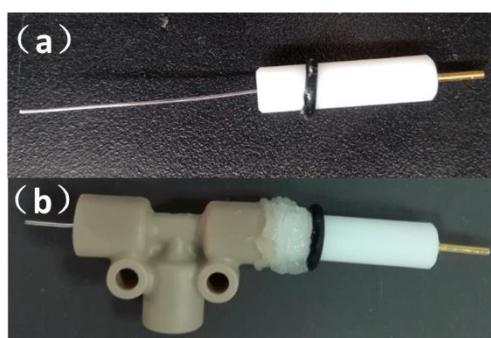
Figure 2. Pt wire (a) was resealed (b).
