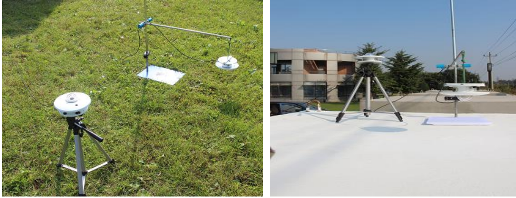
Figure 3. Photos for field tests of ground albedo and roof albedos on two clear calm days (September 20 and 21, 2013).
