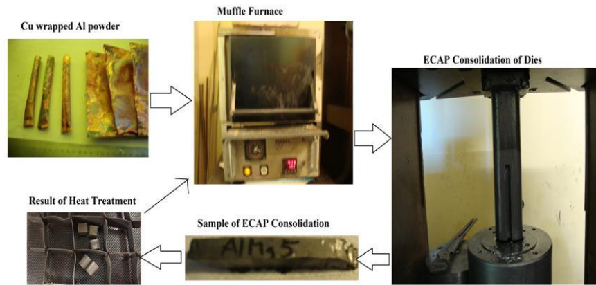
Figure 2. The preparation process of aluminum-based nano powder ECAP Consolidation
