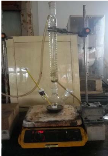
Figure 2. Laboratory scale of leaching limonite
