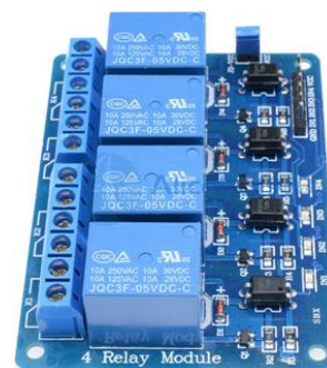
Figure 9. Output relay module with optocouplers and four relay outputs
