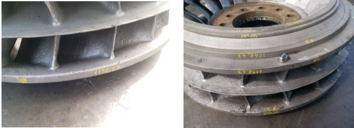
Figure 1. The existing runner with wear marks, high porosity surfaces and cracked areas
