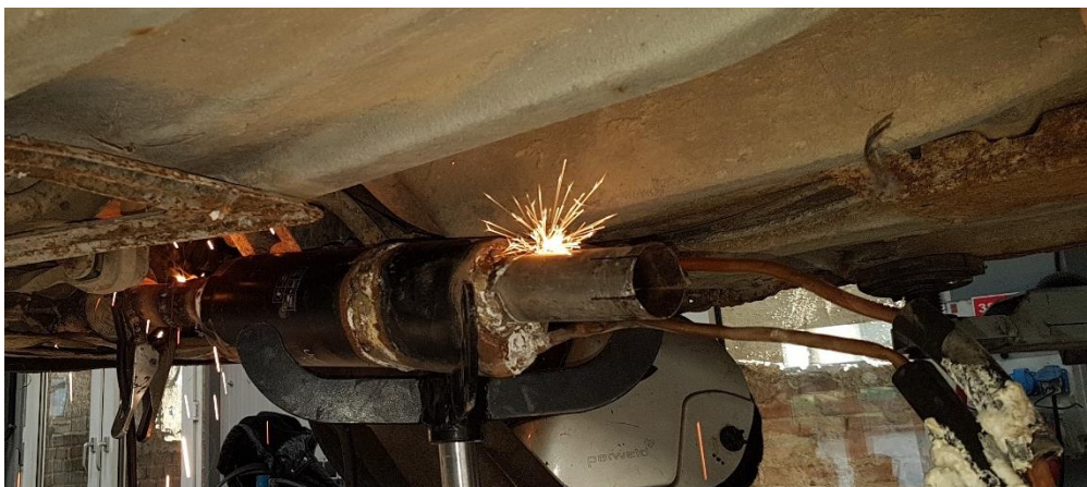
Figure 3. The copper heat exchanger correctly mounted after the catalytic converter
