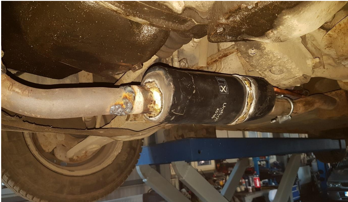
Figure 2. The copper heat exchanger mounted just in front of the exhaust pipe
