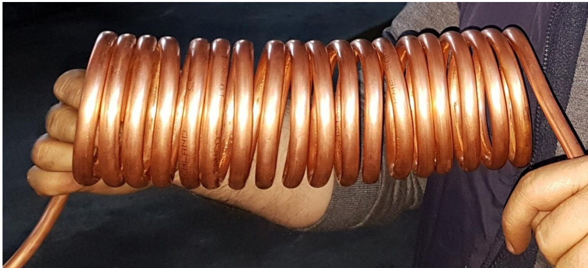
Figure 1. The copper heat exchanger used to recover heat from the exhaust gas
