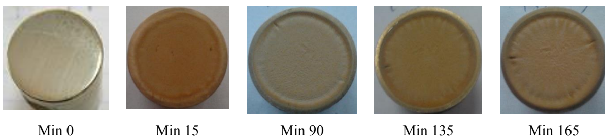
Figure 5. Images of specimen surface at different cavitation exposure time
