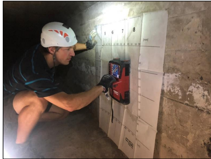
Figure 4. Non-destructive determination of the reinforcement position by radar HILTI PS 1000
