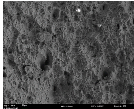
Figure 6. SEM of fatigue crack in specimen.
