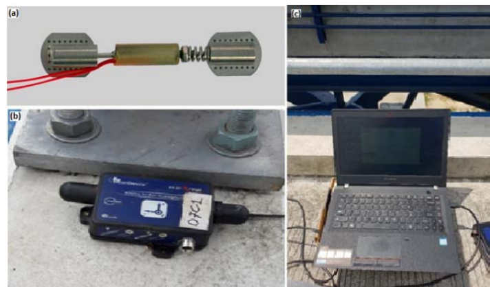
Figure 2. (a) Vibrating Wire Strain Gauge; (b) Vibration Sensor; (c) A set of Laptop.
