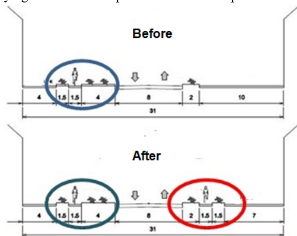
Figure 3. Rebuilding of street a cross-section by reducing the width of the sidewalk and construction of a one-way bike- path, width 1.5 m, and a lane separating the bike path from the carriageway 2 m and a strip separating from the sidewalk, 1.5 m wide [3]
