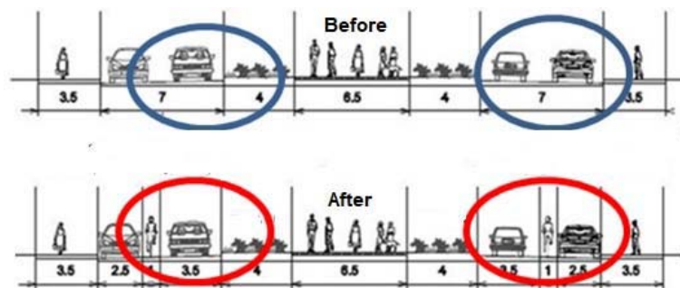
Figure 6. Transforming the street cross-section by changing the use of extreme lanes for parallel parking lanes and lanes for bicycles on the carriageway. Pedestrian traffic is on the sidewalks along the building line and on the promenade on the central belt [3].
