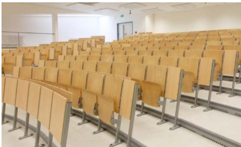
Figure 3. Big lecture hall with circular perforated openings for supply air
