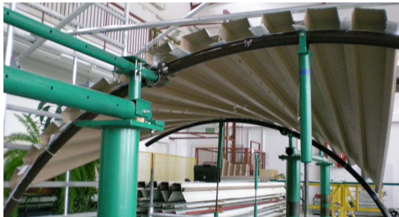
Figure 1. Corrugated shell sheets spread on straight and curved directrices.
