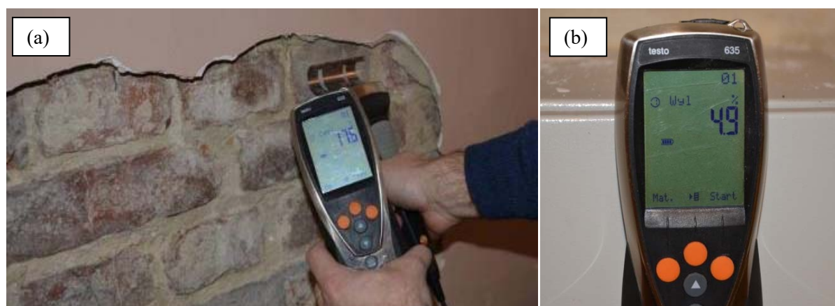
Figure 1. Measurement of mass humidity of the brick (a) and (b)
