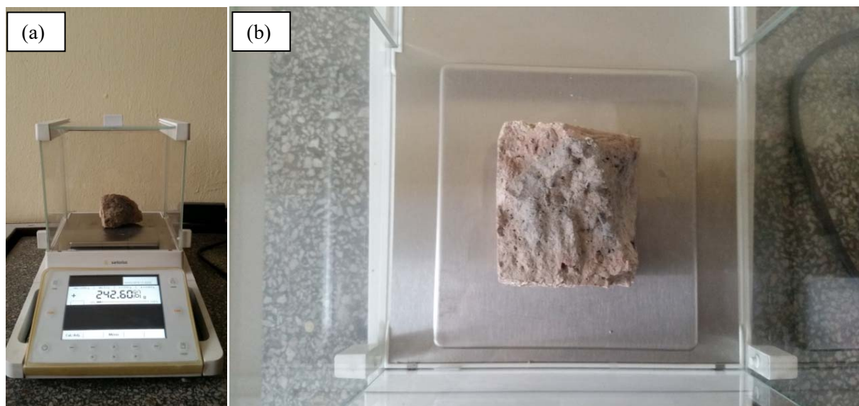
Figure 5. Testing of the sample in the moisture analyser (a) and (b)
