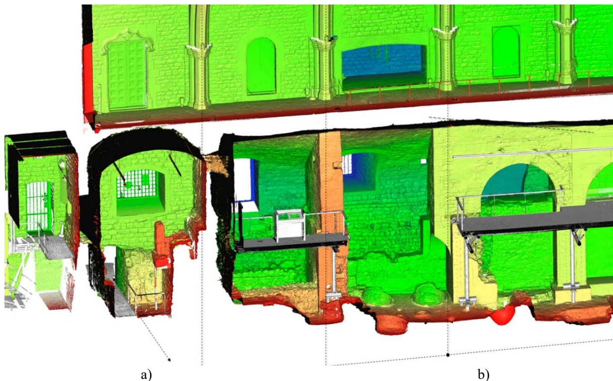
Figure 6. Axonometric detail of a longitudinal section. a) Remains of an external circulation, b) Change in the modulation of the structure (arches and vaults) and point of inflection between changes of slope of the vault.
