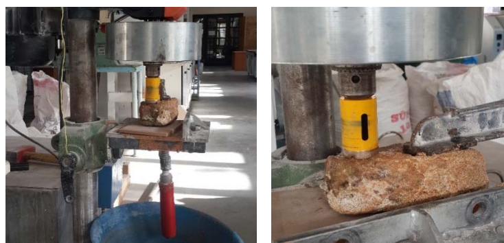
Figure 6. Coring from stone sample
