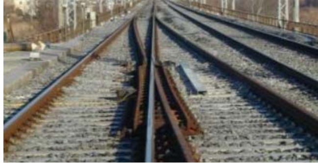
Figure 12. A typical movable crossing [30]
