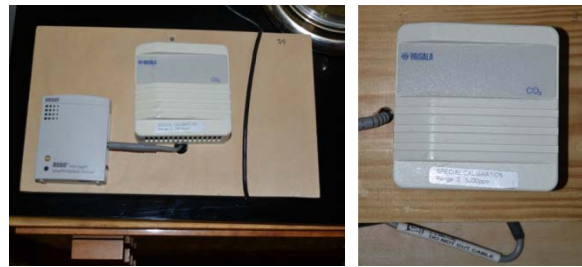
Figure 4: Hobo data logger and Carbocap CO 2 monitor
