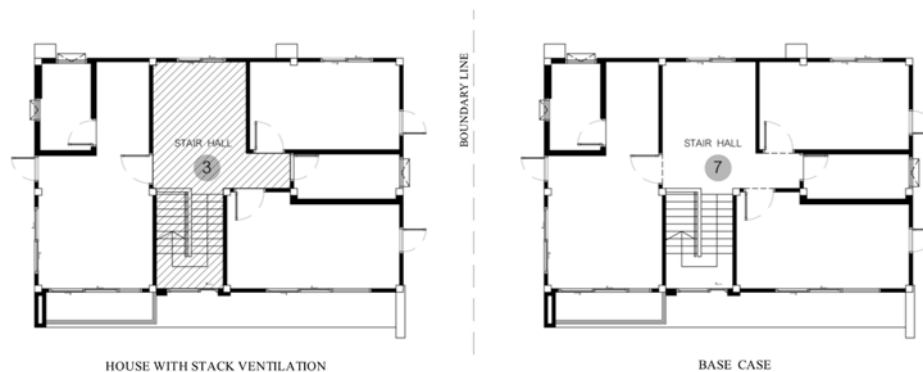
Figure 5. Position of temperature and relative humidity data loggers at 1-meter height above second floor. Shaded areas indicated stack ventilation
