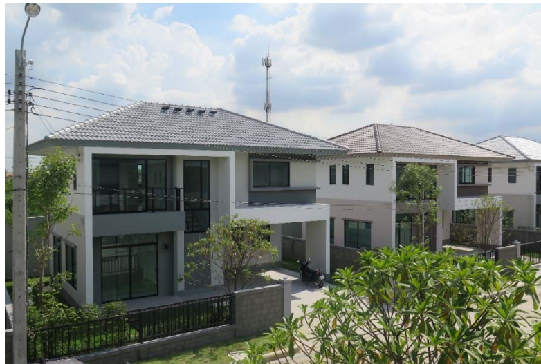
Figure 1. Two houses facing north in the experiment. The house on the left hand side had stack ventilation while the house on the right hand side was a typical house used as a base case.
