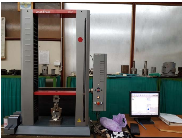
Figure 3 – Testing machine for compression
