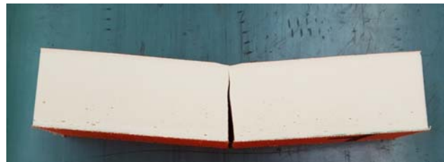
b) Failure of the tension face
