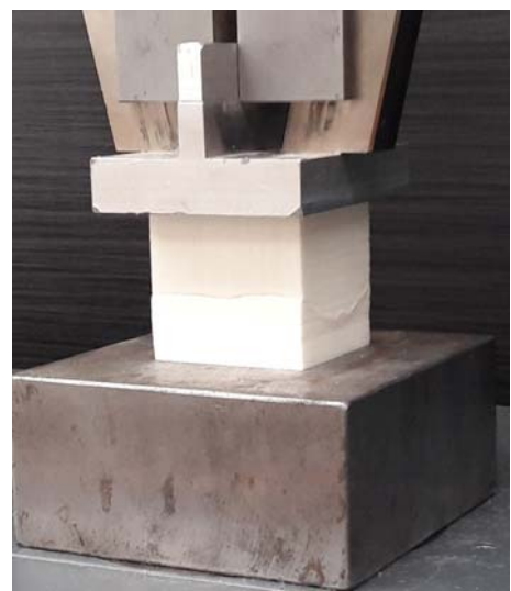
Figure 2 – PIR foam samples for compression test
