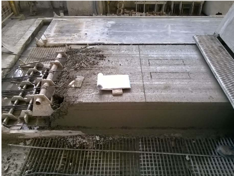
Figure 1. View of a moulded face of an element on a prestressing bed with a marking of the cutting line and technological openings
