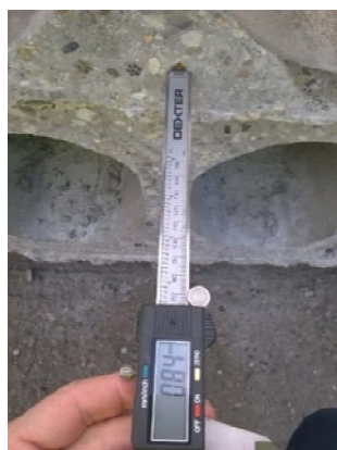
Figure 5. Measurement of strands slip on a forehead of “HC” slab
