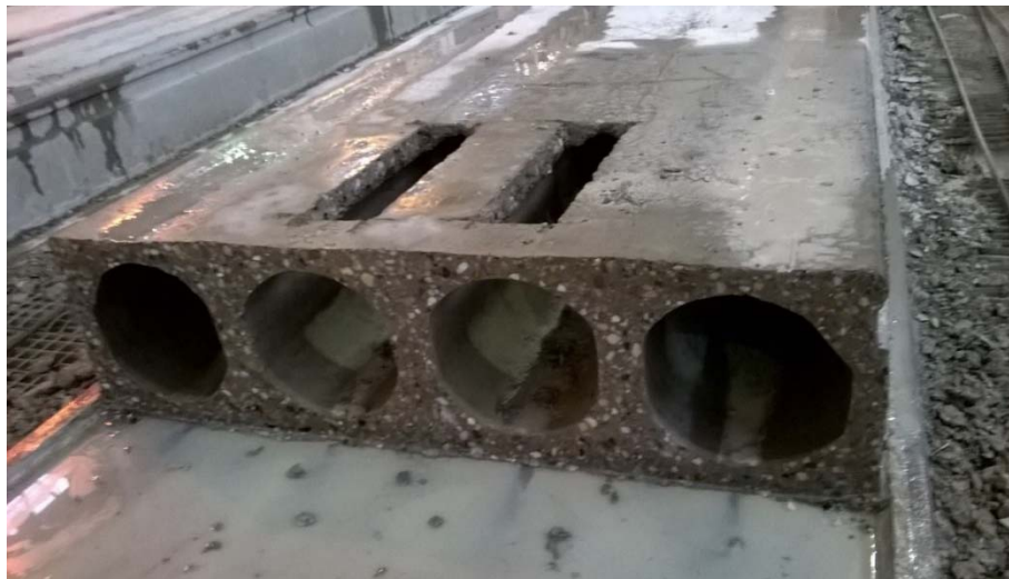
Figure 3. Face of a slab "HC 320" after cutting on a prestressing bed
