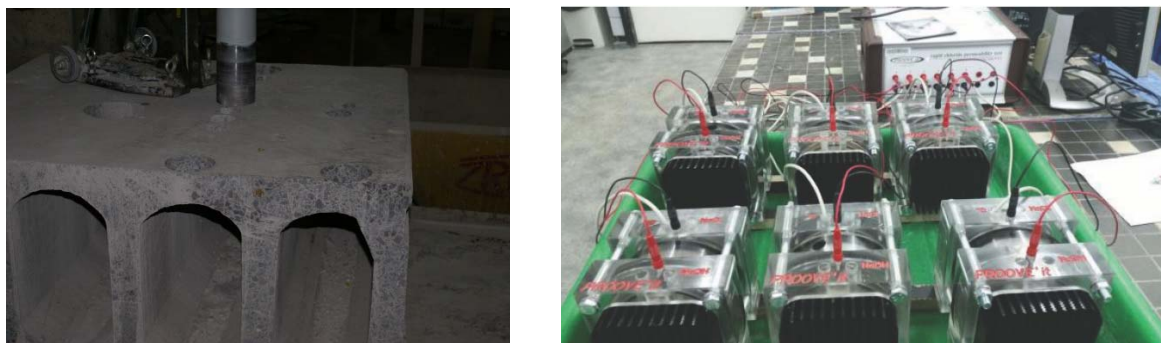
Figure 1. (Left) Sampling of concrete specimens from HC500 floor slabs. (Right) Migration laboratory setup for tests ASTM C 1202-97 [3] of concrete specimens [15].
