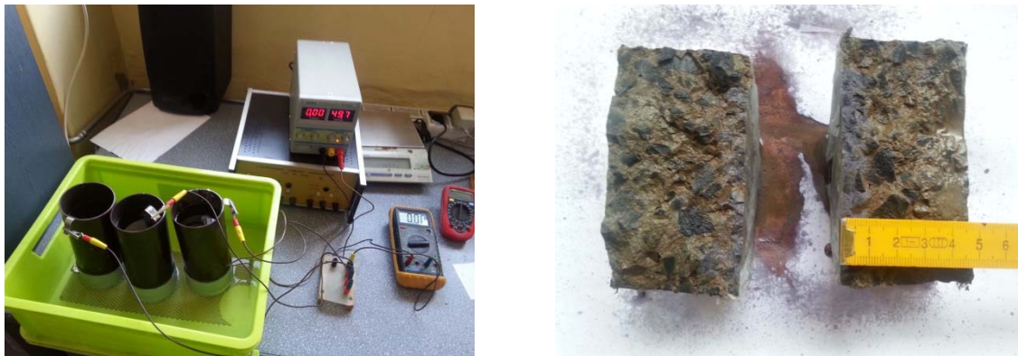
Figure 2. (Left) Migration laboratory setup for tests NT-Build 492 [4] of concrete specimens. (Right) Depth of chloride penetration x_d determined with the colourimetric method
