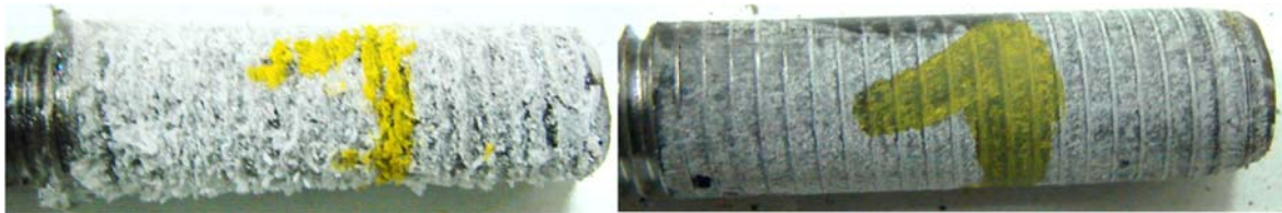
Figure 6. Epoxy 531 (left); 531-C10 (right), specimens after failure.
