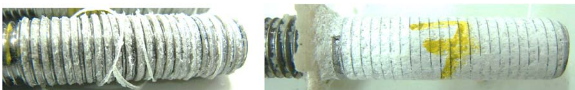
Figure 4. Derakane 411 (left); Derakane 411-V80 (right); specimens after failure
