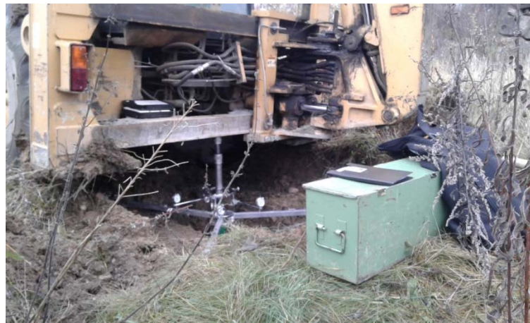
Figure 6. Static plate test performed for road improvement design
