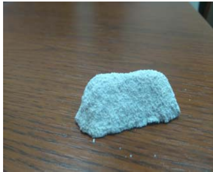
Figure 4. Traditional sand-lime brick. Broken off part of the material.
