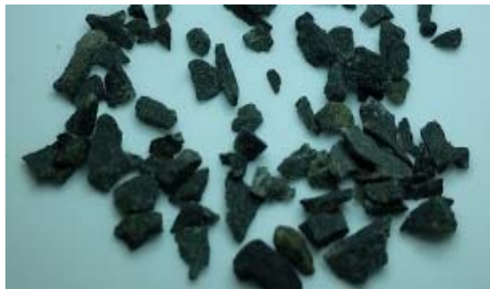
Figure 7. Diabase aggregate used for modification of sand-lime bricks.
