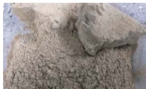
Figure 6. Barite aggregate used for modification of sand-lime mass (particle size up to 2 mm).
