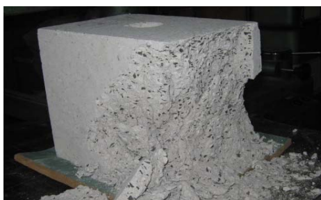
Figure 5. Acoustic brick modified by basalt aggregate (grain size up to 2 mm).
