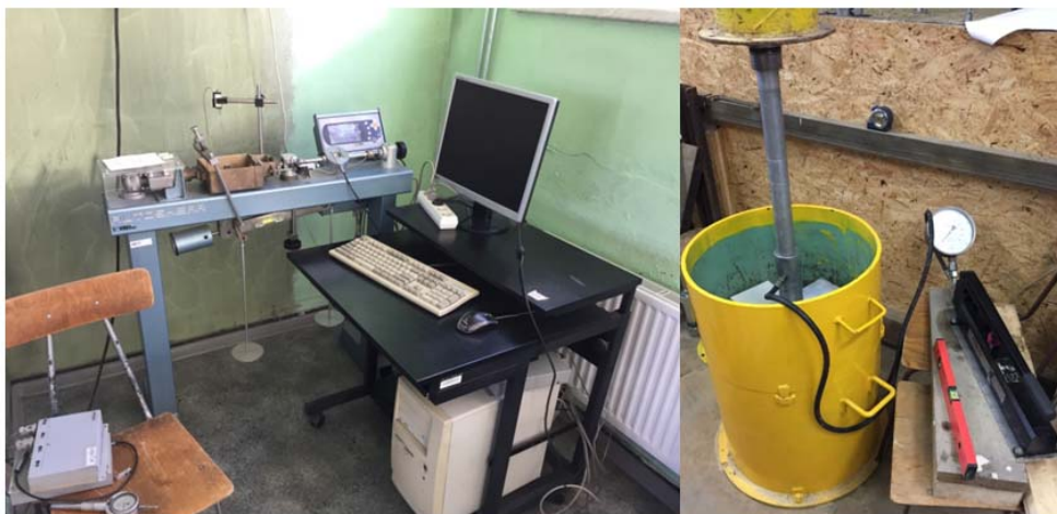
Figure 1. Direct shearing apparatus test stand (left) and small-scale trial loading test stand (right)
