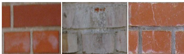
Figure 1. Efflorescence types: a) deposit, b) sediment, c) infiltration
