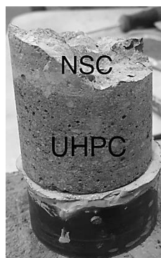
Figure 10. Fractured substrate in grooved direct tension specimen
