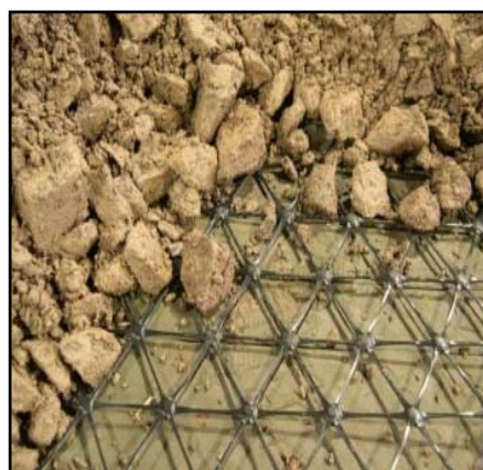
Figure 4. Stiff geogrid with interlocked stones
