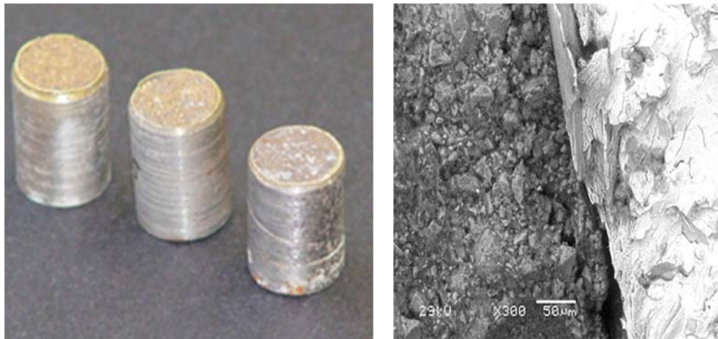
Figure 3. Sleeves filled with mortar after fracturing. Notch edge in the top part of the sample can be seen on the photo. Contact magnification on the adjacent photo
