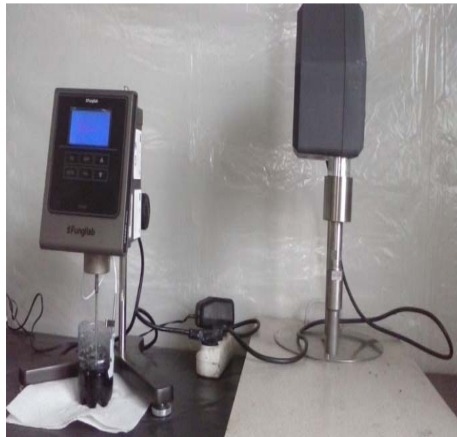
Figure 1. The test stand – the sonicator and rotational viscometer.
