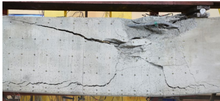
Figure 3. Failure of the beam
